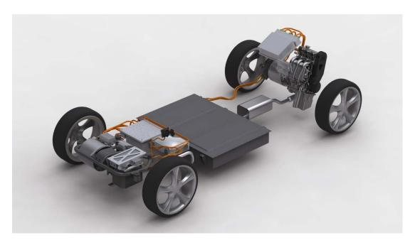
rive is assured by an electric motor with continuous power of 45 kW and 75 kW peak power.
