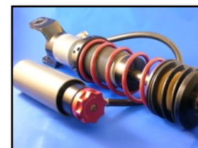
Multi-Pro Suspension developed by Eibach and Callaway. Ten position adjustable compression & rebound kits from $2995
