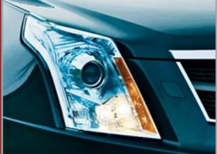
**Adaptive Forward Lighting**, an available feature, uses sensors to read speed and steering angle, and swivels high-intensity headlamps up to 15° to follow direction of travel.
