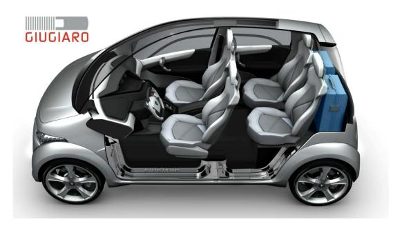
The lower part of the central console, housing the ignition button and gear selector, extends towards the tunnel and can be folded down. When parking in a tight spot, forcing the driver or front passenger to leave the car from the opposite side, this central element can be lowered and the seat moved back so that they can get out on the other side without hindrance.
