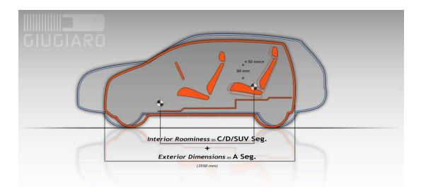
"These new PROTON cars are higher than other compact car models to make the best use of interior space; the seat H point is at the same height as the passengers' hips: you do not get down into your car as in a coupé, you do not climb up as in an SUV but you enter in a natural way. Rear seat comfort when you enter and leave the car is absolutely unprecedented, the distance from the front seat is comparable to that of an SUV", added Giugiaro.
