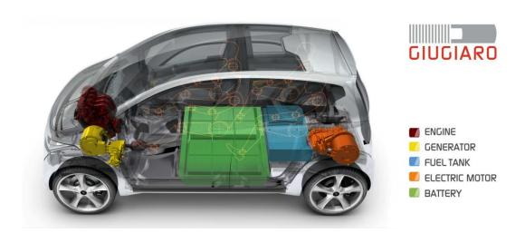
The platform, specially designed by Italdesign Giugiaro for this car family, includes a raised floorpan that is able to accommodate the hybrid or electric system batteries in the centre. The raised position of the seats, all electrically adjustable, allows passengers to make the best possible use of the interior space.
