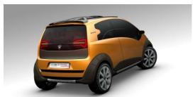
Access to the car is still easy due to generous doors measuring no less than 1350 mm in length and the ergonomic and rational position of the rear seats, that are set 120 mm further forward than in the five-door version.
