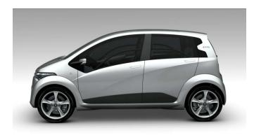
**Emas Comfort**: hatchback saloon, five doors, four seats, length of 3550 mm, hybrid drivetrain in **Comfort**
