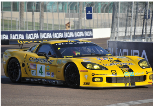
The two Corvette C6.Rs in the GT1 class are powered by E85 fuel. (AMERICAN LE MANS SERIES)
