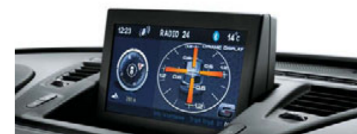
Radio NAV also shows the acceleration value (longitudinal and lateral) the car is subject to. (G-Force meter).
