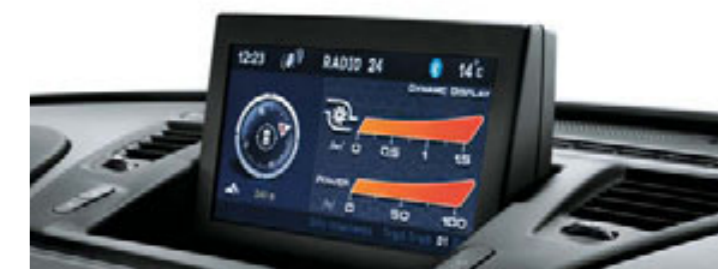
Radio NAV shows turbo-charging pressure and power delivery.
