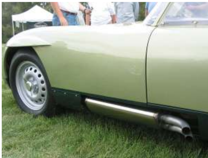
Custom stainless steel muffler built to the original MG engineering drawings.
