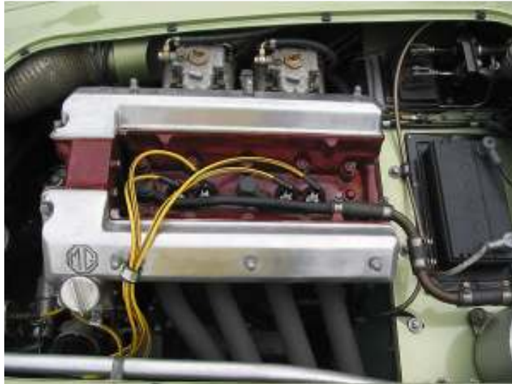
Dual Weber 42DCOE two-barrel, side-draft carburetors. EX186 was never equipped with S.U. carburetors.
