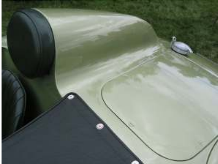
LeMans rules required that all cars be fitted with a spare tire. EX186's was located under this cover.
