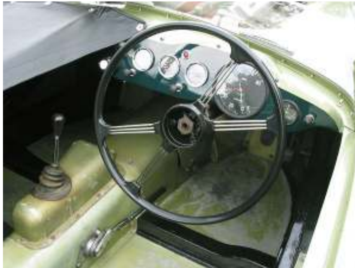
A stock MGA steering wheel was utilized, albeit with the center removed.
