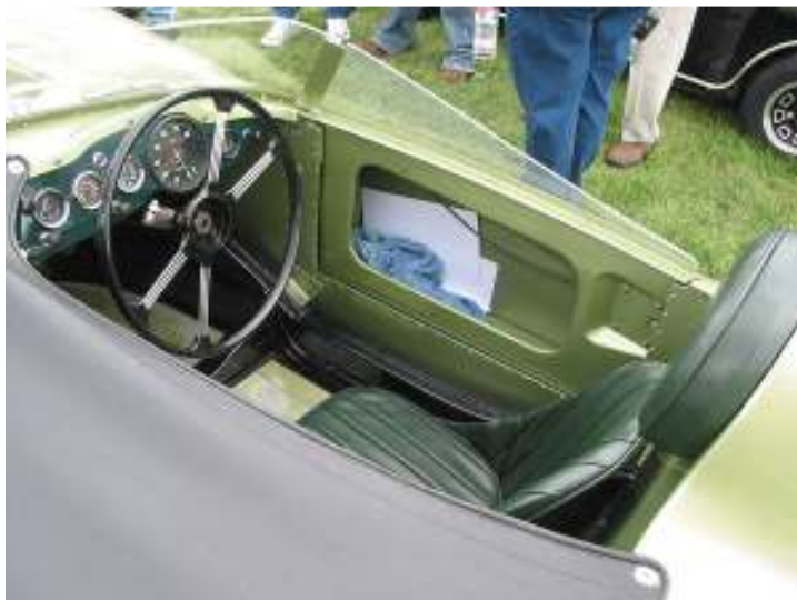
EX186 is a well-crafted car. The custom aluminum doors feature special aluminum hinges, but they utilize standard MGA latches. The doors fit properly, and open and close quite neatly.
