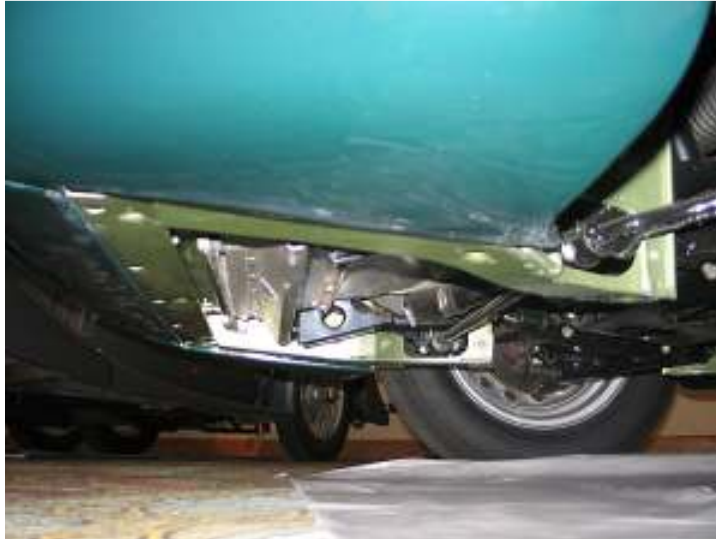
Smooth aluminum panels the full length and width of the bottom of the car minimized aerodynamic drag. Known as "bellypans", these panels are easily removeable for access to engine and suspension. (Here, and in the next three photos, bellypans have been temporarily removed for our inspection.)
