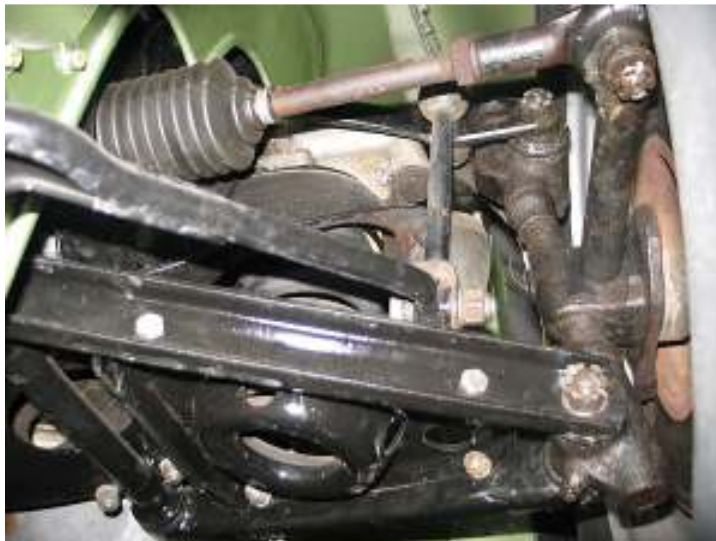
EX186's front suspension is similar to a stock MGA Twin-Cam. Differences include an all-aluminum steering rack, noticeably different upper control arms, and lightened lower control arms.
