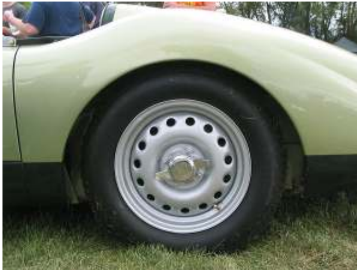
15x5.5 Dunlop peg-drive knock-off steel wheels. Dunlop bias-ply historic racing tires.
