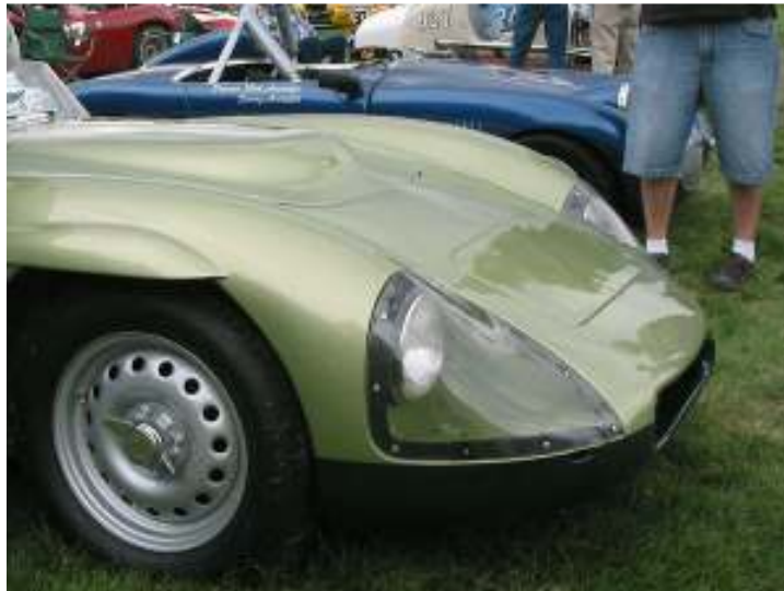
EX186 is shown here with its original Perspex headlamp covers, not reproductions.
