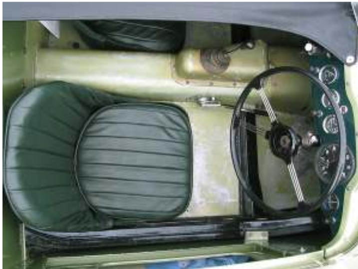
Left to right: Jaeger fuel level gauge, Smiths oil temperature gauge, Jaeger dual oil pressure/coolant temperature gauge, Smiths chronometer ("tachometer") with tattletale, and Lucas amp gauge.
