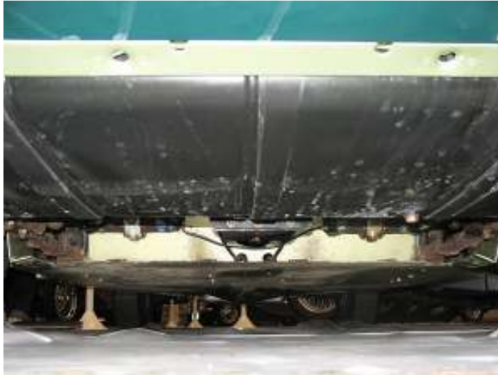
From the rear, with bellypan removed, you can see the fuel tank and twin S.U. fuel pumps. (You can also see eight of the Dzus fastener receptor springs that would secure the bellypan.)
