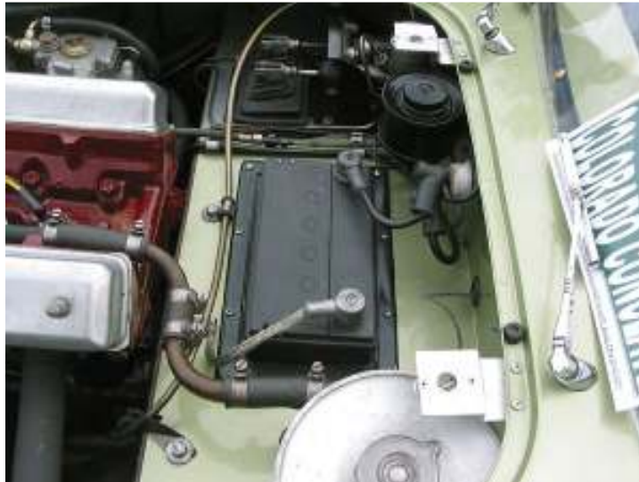
Foreground: the original aluminum coolant swirl tank is used for de-aeration. Center: a modern Suzuki battery fits neatly in the original battery's location.
