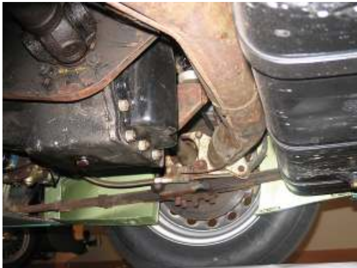
The rigid transverse beam of a deDion rear suspension keeps the rear wheels parallel in all situations. Compared to a stock MGA, the rear springs are relatively soft. No rear anti-sway bar is employed.
