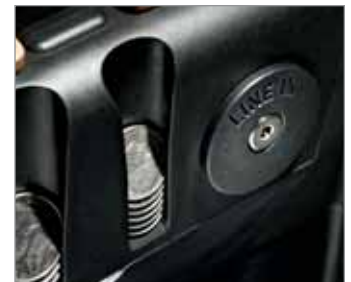
A standard audio input jack allows plug-and-play capability with your digital media player.
