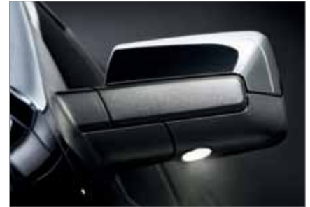
Power-folding heated sideview mirrors feature security approach lamps that activate when your key fob is pressed.
