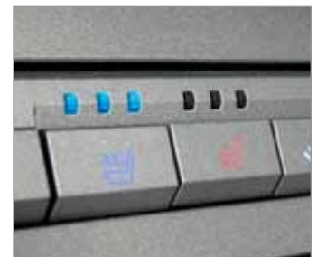
Standard heated and cooled front seats have three levels of warming or cooling power.
