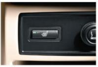
☐ Seat heating at the rear: Same as the electric heating of the driver's and front passenger's seats, with heating in two stages, available in conjunction with leather upholstery.
