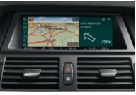
□ Navigation system Professional\* with colour 8.8-inch display, traffic guidance provided by voice information, arrows and street maps. The split-screen function allows you, for example, to view radio and navigation data simultaneously.
