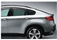
☐ Sun-insulating glass for the rear side windows (behind the B-pillar) and rear window; these tinted windows reduce sun glare and ensure a pleasant temperature inside the car even in hot weather.
