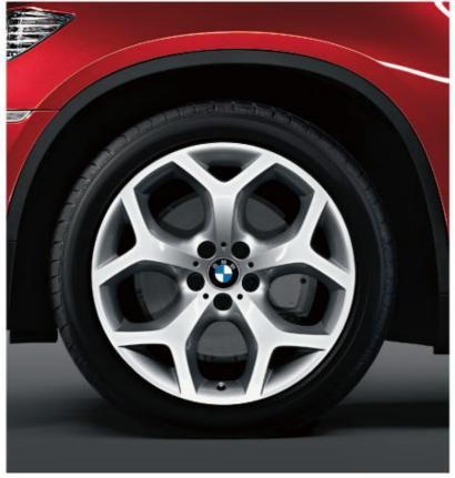
☐ **BMW light-alloy wheels Y-spoke 214** with mixed and runflat tyres, 10 J x 20-inch at the front on 275/40 R 20 tyres, 11 J x 20-inch at the rear on 315/35 R 20 tyres.
