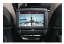
□ DVD system in the rear offers an independently controllable DVD player with a fold-down 8-inch screen. The system can be operated by wireless remote control, has sockets for two headphones and a video source, and is compatible with infra-red headphones. In conjunction with the TV function, the same TV programme can be viewed simultaneously on the front (at a standstill) and rear screens.
