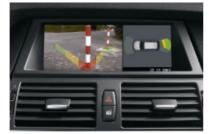
☐ Rear view camera clearly shows the area behind the vehicle on the Control Display, where interactive road line markings show for example, whether the target parking space is large enough for the vehicle. The rear view camera is activated automatically when the reverse gear is selected.
