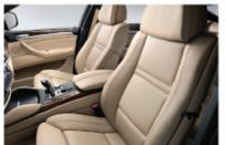
□ Comfort seats for driver and passenger. The seats have comfort head-restraints with electrically adjustable head-restraint height and mechanically folding side bolsters. The thigh support and upper seat back are also electrically adjustable, as is the seat height.
