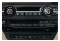
■ Functional bookmarks: With these buttons, the driver and passenger can save their most frequently used navigation, audio (e.g. certain radio stations or CD tracks) or telephone functions on eight separate buttons for rapid access.
