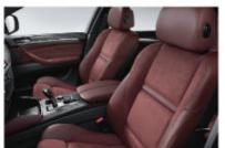
☐ Sports seats for driver and passenger, highly contoured seat sides for optimal lateral support. Seat height, seat angle and backrest angle are electrically adjustable, thigh support manually adjustable. The driver's seat, driver's head restraint height, exterior mirrors and steering column feature a memory function.
