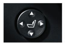
□ Lumbar support on driver's and front passenger's seats, electrically adjustable for height and depth, to provide a perfectly ergonomic seating position and support your back muscles.
