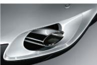
**Tailpipes:** The X6 xDrive35i, X6 xDrive30d and X6 xDrive35d models come with two single tailpipes. The exhaust system is made of high-quality stainless steel. The visible tailpipes are trimmed with a chrome surround.
