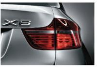
■ Dynamic Braking Lights make it easier for drivers following from behind to see how hard you are applying the brakes. If you are braking normally, the brake lights cover a larger area; only during emergency braking do the brake lights start to flash. This allows following traffic to distinguish between a slight tap on the brakes and full braking – for even greater safety on the road.
