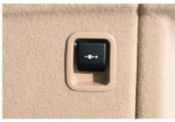
■ Sockets (12-V), one in the front storage box, one in the rear centre console and one in the luggage compartment.
