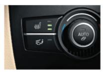
☐ Seat heating for driver and front passenger: Seat surfaces and backrests with heating in three stages for pleasant temperatures shortly after setting off.
