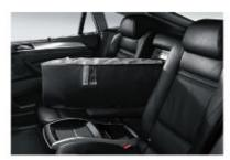
☐ **Ski bag** for clean and safe transport of up to four pairs of skis with up to four occupants in the car; whenever the ski bag is not required, it remains stored conveniently and out of sight behind the centre armrest.
