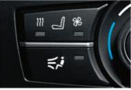
□ Active seat ventilation provides a noticeably more comfortable ride. Fans in the seat base and backrest blow air through the seat covers (available for the driver and passenger in conjunction with Nevada leather, perforated and comfort seats).
