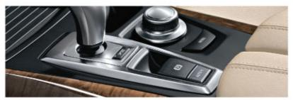
■ Parking brake with Auto-Hold function provides the convenience of being able to hold and release the vehicle by means of a button in the central console.
