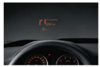
☐ Head-Up Display shows relevant information, for example current speed, directly in the driver's field of vision. Arrow directions for navigation, for instance, can also be shown. Height and brightness of the display can be individually adjusted, so that the driver can fully concentrate on the traffic at all times.
