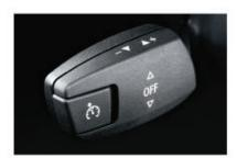
■ Cruise control with braking function facilitates comfortable driving at a pre-selected speed (30–250 km/h).
