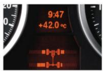
■ Dynamic Performance Control Display in the instrument panel. Shows the distribution of drive by xDrive between the front and rear axle, and the flexible distribution of power between the rear wheels by Dynamic Performance Control.
