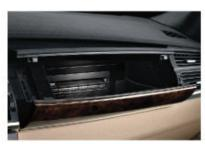
☐ **CD changer**, 6-disc single slot changer, with features including scan function, random play and MP3 decoder; installed in the glove compartment.
