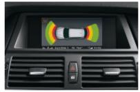
☐ Park Distance Control (PDC), front (standard at the rear), makes parking and manoeuvring easier in the narrowest spaces; the distance between the vehicle and the nearest obstacle is signalled acoustically as well as visually in the Control Display.
