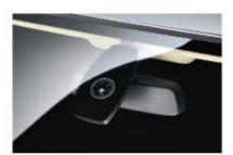
■ Rain sensor incl. automatic driving lights control: Once activated, the rain sensor automatically switches on the windscreen wipers and controls wiper frequency, depending on how hard it is raining. This feature includes automatic driving lights control switching on the low-beam headlights automatically, for example, when it gets dark or when entering a tunnel.
