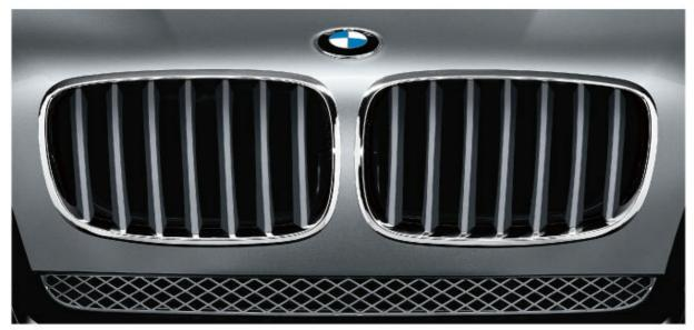
Front ornamental grille with titanium-coloured slats in the kidney grille and chrome surround (standard on the X6 xDrive50i and X6 xDrive35d). (Shown here in combination with the sports package; with radiator grille in contrasting colour).
