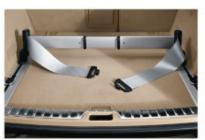
☐ Adaptive fastening system for firmly securing differently-sized pieces of luggage (available in combination with the storage compartment package.)
