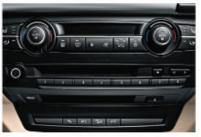
■ Radio BMW Professional, 4-channel amplifier, 2-tuner reception, antenna diversity, scan function, CD player, MP3 decoder, 6 loudspeakers.
