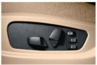
☐ Seat adjustment, electric, of driver's and front passenger's seats, with memory function for driver's seat, steering column and exterior mirrors, including easy access (standard on the X6 xDrive50i and X6 xDrive35d).
