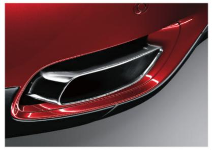
**Tailpipes:** For the X6 xDrive50i model the exhaust system with two rectangular tailpipes is made of high-quality stainless steel, the rear ends are bordered with a chrome surround.
