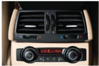
□ 4-zone automatic air conditioning. As for 2-zone air conditioning, plus the climate in the rear area of the vehicle can be separately controlled with two dials and a display. This feature includes an additional blower and footspace air outlet in the rear.
