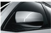
■ Exterior mirrors, electrically adjustable and heated, finished in body colour (mirror foot in black), in aspheric design and blue-tinted.
