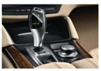
■ Six-speed automatic transmission with Steptronic. Gears are shifted very quickly and smoothly for optimum performance.
