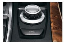
■ Controller is the central iDrive input element (for driver and passenger). Additional functions can be activated from the Control Display using this rotary/push button. Menu navigation is oriented to the four cardinal points. Four different menus are available: Climate, Communication, Entertainment and on-board info (optional navigation).
