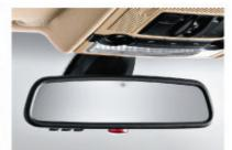
□ Interior mirror and exterior mirror, with automatic anti-glare function which activates once a certain light intensity from following vehicles is reached. With fold-in function for exterior mirror.
