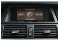
■ Control Display with TFT screen (6.5-inch, colour). Shows the functions activated by the Controller (e.g. on-board computer or radio). In conjunction with the optional navigation system Professional\* or with the TV function, the screen measures 8.8 inches.
