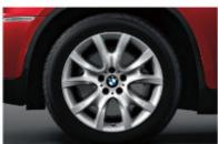
☐ BMW light-alloy wheels **V-spoke 257**, 9 J x 19-inch with 255/50 R 19 runflat tyres (standard for X6 xDrive50i).
