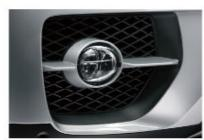
■ Fog lights in free-form technology, integrated in the front air dam, ensure extra safety in poor visibility.
