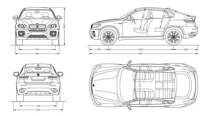
All dimensions of the technical drawings in millimetres. Hight includes roof antenna. Luggage compartment capacity (VDA method) 570 –1,450 litres.
