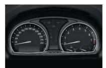
■ Instrument panel with analogue-face instruments with red illumination from behind, speedometer with LC display for mileage and trip counter, on-board computer, rev counter with integrated fuel gauge and coolant thermometer.
