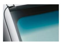
□ Climate comfort windscreen, this useful amenity reduces the temperature within the car by means of an infra-red light-reflecting layer, the green stripe at the top of the windscreen removing any direct sun glare.
