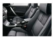
Sports seats for driver and front passenger. Generous bolsters for optimum lateral support at all times. Individual adjustment of seat height, inclination and longitudinal position, backrest angle and thigh support.
