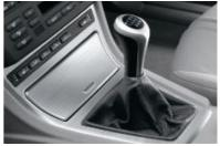
■ 6-speed manual transmission makes for extremely dynamic driving. Smooth and optimally synchronised, it boasts precise, tight throw gear shifts. Thanks to the wider ratio transmission with an additional sixth gear the engine is even more responsive to your own personal style of driving (not available on X3 xDrive35d).
