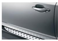
☐ **Aluminium running boards** made of brushed and eloxy-plated aluminium with rubber inserts.
