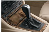
☐ 6-speed automatic transmission with Steptronic, Adaptive Transmission Management (ATM), Shiftlock/Interlock. For exceptionally smooth and agile gear changing, and unsurpassed driving dynamics (standard on X3 xDrive35d, not available for X3 xDrive20i).
