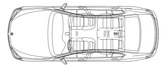
All dimensions in the technical drawings are given in millimetres. Luggage compartment volume 500 litres. Figures in () refer to 7 Series short-wheelbase version.
