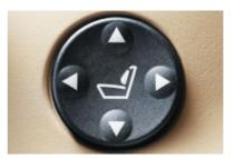
☐ **Lumbar support** for driver and front passenger seats, electrically adjustable vertically and horizontally, for an ergonomically sound seating position and added back muscle support.
