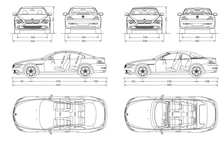
All dimensions in technical drawings given in millimetres. Luggage compartment volume, BMW Convertible: approx. 300 litres (350 litres with raised soft top compartment, VDA measurement); BMW Coupé: approx. 450 litres (VDA measurement).
