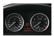
■ Info Display with precise, anti-glare analogue instruments. Information such as time, exterior temperature and trip mileage can be selected at any time on LC displays in the instrument panel.
