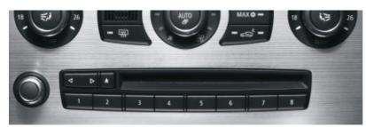
■ Functional bookmarks: Each button can be programmed to instantly activate any commonly-used function of the navigation, audio or telephone systems, (e.g. a radio station or a CD title), enabling the driver and front passenger to access eight favourite functions with ease.
