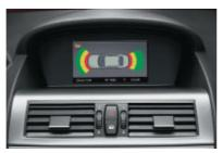
☐ Park Distance Control (PDC), front and rear, aids parking and manoeuvring in tight spaces. The proximity of obstacles is indicated acoustically and visually in the Control Display.
