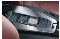
☐ Mobile phone preparation with Bluetooth interface (incl. hands-free facility, charger connection and aerial). A Bluetooth-compatible phone can be connected using a snap-in adapter (separately available), allowing control via the multifunction steering wheel and voice control system. Your local BMW partner will be happy to advise on recommended telephones.
