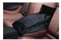
☐ **Ski bag** enables up to two pairs of skis or one snowboard to be transported even when every seat is occupied. When not needed, the ski bag is stored in the centre armrest, out of sight.
