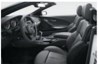
Sports seats for driver and front passenger with memory function for driver's seat feature pronounced side bolsters for excellent lateral support in every driving situation; seat height, cushion angle, backrest angle and fore-and-aft position are all individually poweradjustable. The thigh support is manually adjustable. Lumbar support is standard in connection with the M leather steering wheel, the perfect combination of dynamics and comfort.
