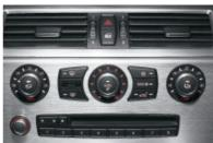
■ Automatic air conditioning with extra features, including Automatic Air Recirculation (AAR), solar and condensation sensors, automatic temperature control, air distribution (separate for driver and passenger) and airflow control. Settings shown on Control Display.
