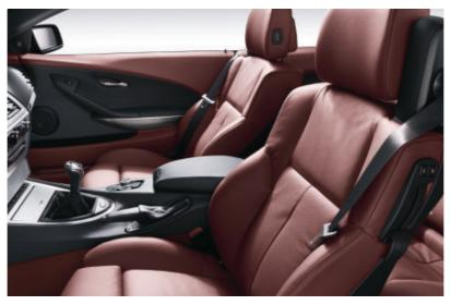
□ Sports seats for driver and front passenger, incl. memory function for driver's seat (the BMW 6 Series Convertible with Dakota leather upholstery shown here). Pronounced side bolsters ensure optimal lateral support in all driving conditions. Electric adjustment of height, length, backrest angle and tilt control. Thigh support manually adjustable. With lumbar support as standard.
