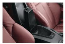
■ Front armrest, two height positions, including storage bin (shown here) for small items. (Storage bin located under telephone unit when combined with mobile phone preparation).
