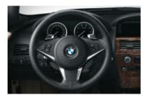
■ Sports leather steering wheel, three spokes, with multifunction; the driver can operate radio, CD player and telephone (optional) via integrated buttons – keeping both hands safely on the steering wheel.
