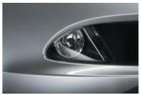
■ Fog lights built into the front air dam, improving safety in poor visibility conditions. Ellipsoid freeform technology enables very even illumination of the road.
