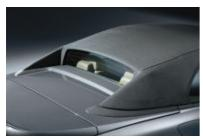
■ Fin roof, fully-automatic. Sets unprecedented standards in noise insulation. In connection with the retractable rear window, it offers very effective ventilation of the vehicle interior. When closed, it gives the convertible a typical coupé-like silhouette; when opened, it is stowed in the soft top compartment fitted in the luggage compartment. Available in grey or black.
