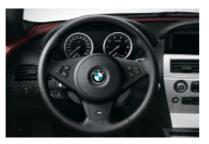
☐ M leather steering wheel, rim designed for optimal grip, three spokes, with multifunction; the driver can operate radio, CD player and telephone (optional) via integrated buttons – keeping both hands safely on the steering wheel.
