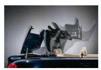
■ Fully-automatic roof operation: the open/ close function occurs automatically at the touch of a button (when vehicle is stationary). The vertical rear window can be retracted independently of the soft top. The soft top can also be opened comfortably via the radio remote control.
