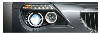
■ Xenon Headlights for high and low beam, with automatic headlight range control, significantly improve road illumination at night, in bad weather or poor visibility. In combination with the optional Adaptive Headlights with variable light distribution, they illuminate bends via electromechanical movement of the headlights when the driver turns the steering wheel.
