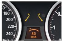
☐ The Lane Departure Warning system uses a camera to monitor when the vehicle is approaching lane markings, and immediately warns the driver via a steering wheel vibration. The system is designed for country roads and motorways, and is switched on and off with a button in the multifunction steering wheel.
