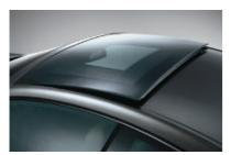
☐ Glass roof, with electrically operated lift function and sun shade, and comfort opening / closing via tip keys.
