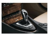
☐ 6-speed sports automatic transmission offers a particularly sporting transmission character with faster gearshifts for an even more dynamic driving experience; gearshift paddles are mounted on the sports leather steering wheel. (Standard for 635d)
