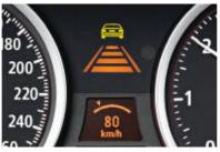
☐ Active Cruise Control with Stop&Go function. Driving assistance system for increased comfort and active safety in particular for driving in slow-moving traffic. Combines Cruise Control with active safe distance control to a stand-still in bumper-tobumper driving, with automatic restart in typical "stop and go" situations.
