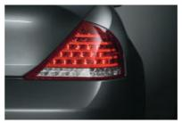
■ Brake Force Display helps following drivers to judge your braking situation. Under light braking, the lower three rows of LEDs in the rear light units illuminate in red, along with the light guide strips of the rear lights whenever driving lights are not in use. Under full braking force, the upper two rows of LEDs also illuminate, generating especially bright braking light.
