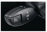
■ Cruise Control with braking function lets you store and maintain a chosen speed above approx. 30 km/h (activated by lefthand control stalk on the steering column). After accelerating, the pre-selected speed is automatically resumed.
