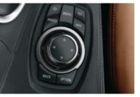
■ Controller, the core element of iDrive (for driver and front passenger), is a rotary/push button for controlling a multitude of functions via the Control Display. The new direct menu control buttons open the menu for the CD, radio, navigation system\* and telephone; tactile design ensures each key can be identified through touch alone.
