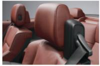
■ Seat-integrated belt system for the BMW 6 Series Convertible provides optimal passenger protection and ideal seatbelt ergonomics in every position.
