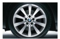
$\square$  BMW light-alloy wheels styling 218 with mixed runflat tyres, 8.5 J x 19" wheels with 245/40 R 19 tyres at the front, 9 J x 19" wheels with 275/35 R 19 tyres at the rear.
