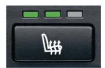
☐ Seat heating, for driver and front passenger. With heated cushion and backrest, providing comfortable warmth quickly after beginning the journey (standard on 650i).
