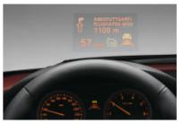
☐ **Head-up Display** conveys important information such as current speed directly in the driver's field of vision. Direction arrows from the navigation system, Active Cruise Control functions and Check Control data can also be displayed.
