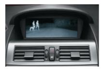
□ BMW Night Vision uses an infrared camera to detect people and animals beyond the scope of the headlights at a distance of up to 300 metres. The camera's image appears in the Control Display, enabling you to avoid danger in good time on poorly lit roads.
