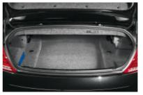
■ Luggage compartment, with soft-top compartment raised: When the soft-top is closed the soft-top compartment is not required and can be easily moved forwards and raised with one hand. The spacious and easily-accessible boot is thus fully available for luggage.
