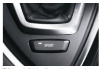
■ Dynamic Driving Control (sport mode), at the touch of a button, engine response to the accelerator becomes even more spontaneous. In models with sports automatic transmission shift times are shorter and up-shifting is delayed for a more sporty driving style. Steering assistance is also reduced for improved feel of the road.
