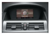
■ Control Display with 6.5-inch colour display. Displays functions selected by the Controller (e.g. on-board computer or radio). Screen size is 8.8-inch in combination with Navigation system Professional\*.
