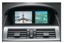
☐ TV function enables the reception of analogue and digital television via the 8.8-inch Control Display when the car is stationary. Can receive terrestrially broadcast and digital (DVB-T) transmissions.
