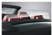
■ Glass rear window, vertically retractable, can be raised and lowered independently of the soft top. When the roof is closed and the rear window is lowered, the interior is effectively ventilated for a pleasant climate. When the roof is open, the raised rear window improves the comfort of rear seat passengers.
