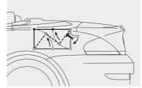
■ Soft top compartment, variable: can be effortlessly raised or lowered with one hand using the integrated swivel handle. The advantage: a special folding mechanism folds the soft top compartment flat, for optimisation of luggage compartment volume. When lowered, the compartment stores the soft top.
