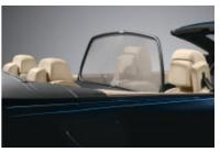
☐ Wind deflector makes open-top driving more pleasurable by reducing irritating drafts and annoying isolated turbulence in the shoulder and neck region. The wind deflector is easy to operate and can be stowed away compactly in the luggage compartment.
