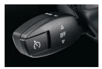
■ Cruise Control with brake function stores any desired speed upwards of approx. 30 km/h and maintains that speed (activated via left-hand control stalk).
