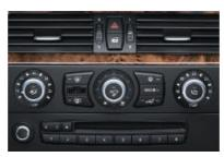
□ Automatic air conditioning, extended with AAR, solar sensor and fogging sensor, automatic temperature control and air distribution (separate for driver and passenger) also air volume control; status and settings shown on the Control Display. With adjustable armrest and air-conditioned storage tray in centre console (standard on 540i, 550i and 535d).
