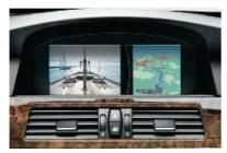
□ **TV function** enables you to use the Control Display as a TV set while the vehicle is stationary. Enables reception of terrestrial analogue and digital (DVB-T) channels.
