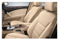
■ Standard seats with manual forward/ backward adjustment, electric seat height and backrest adjustment and manual seat angle adjustment (driver only).
