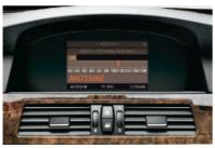
■ Radio Business, 4-channel amplifier, aerial diversity, scan function, CD drive with title scan and automatic CD insert/eject, six loudspeakers and MP3 decoder.
