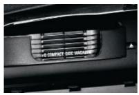
$\square$  **CD changer**, for six CDs, integrated into the glove compartment.
