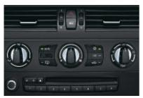
■ Automatic air conditioning with microfilter, enabling you to enjoy your favourite climatic conditions at any time of the year; automatic temperature and air volume control, flap control, ventilation in the rear, status and settings shown on the Control Display.
