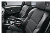
☐ Sports seats for the driver and front passenger provide optimum lateral support thanks to highly contoured seat sides; with individual electric adjustment of seat height and backrest angle, and manual adjustment of seat angle, forward/backward position and thigh support.
