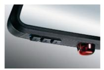
☐ Garage door opener, integrated, provides additional comfort. The self-teaching remote control unit enables you to open and close your garden gate or garage door from within your vehicle.
