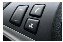
□ Voice control system, enables you to control radio stations, navigation destinations or telephone entries, as shown in the Control Display (this function is part of the navigation system Professional\*).
