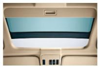
☐ Glass roof, with electric fingertip control for sliding back or raising the roof, trap release and comfort opening/closing function.
