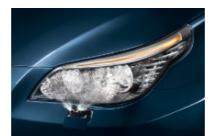
☐ Headlight washing system ensures optimum headlight brightness in all kinds of weather. When the lights are on, the headlights are automatically cleaned in parallel with the windscreen (only in combination with Xenon lights\*).
