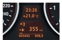
■ Optimum Shift Indicator shows when switching to another gear would be more fuel-efficient. The system recommends when to switch to a higher or lower gear, as appropriate for your driving style. For example, when accelerating, a signal is shown at the point where you could continue to accelerate in a higher gear while however saving fuel (for vehicles with 6-speed manual transmission).
