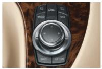
■ Controller: This turn/press button enables intuitive control of different functions shown on the Control Display. Four menus can also be opened via the direct menu control buttons, namely CD, Radio, Navigation and Telephone. Three more buttons, namely Menu, Option and Back facilitate the operation.
