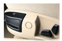
■ Partly electric seat adjustment for driver and front passenger, with electric seat height and backrest adjustment, manual forward/backward adjustment and manual seat angle adjustment on the driver's side.
