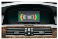
□ Park Distance Control (PDC), front and rear, facilitates parking and manoeuvring in confined spaces; the distance between your car and an obstacle is indicated by an acoustic signal and a visual representation in the Control Display.
