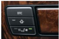
☐ Active seat ventilation enhances summer comfort by ensuring a pleasantly cool seat temperature. Ventilators in the seat surface and backrest blow air through the perforated seat covers. For driver and front passenger seat (only in conjunction with Nasca leather, not in conjunction with sports seats).
