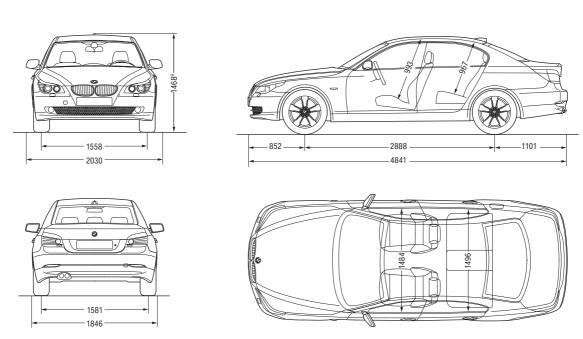
All dimensions in millimetres. Luggage compartment capacity (as per VDA standard): 520 litres (18.4 cu ft).
