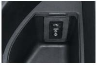
□ **USB/audio interface** allows Apple iPods, MP3 players and USB sticks to be connected for listening to audio files. Operation and playback via the controller, the functional bookmarks, the steering wheel buttons or the relevant audio system.
