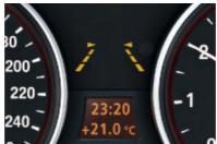
□ Lane Departure Warning System uses a camera to monitor when the vehicle is approaching lane markings, and immediately warns the driver via a steering wheel vibration. The system is designed for country roads and motorways, and is switched on and off with a button in the multifunction steering wheel.
