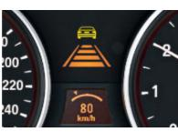
□ Active Cruise Control with Stop & Go function. Driving assistance system for increased comfort and active safety in particular for driving in slow-moving traffic. Combines Cruise Control with active safe distance control to a stand-still in bumper-to-bumper driving, with automatic restart in typical "Stop and Go" situations.
