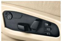
□ Electric seat adjustment for driver and front passenger. All seat planes and headrest height electrically adjustable, with memory function for driver's seat, exterior mirrors and steering column and automatic parking function for exterior mirror on the passenger side (standard on 540i, 550i and 535d).
