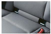
■ ISOFIX child seat fastening system in the rearfor the two outer seats enables easy and safe installation of the optional child seats via locking push connectors.
