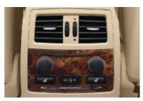
■ Fresh-air outlets at the rear. In conjunction with automatic air conditioning with extended features (shown here), these outlets provide temperature-controlled ventilation of the rear.
