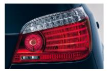
■ Rear light with LED indicators and five radial LED light conductors ensures optimum recognition even in poor visibility. Clear glass sets off this high-quality, modern lighting technology, making for an individual appearance.
