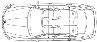
All dimensions in millimetres. Luggage compartment capacity (as per VDA standard): 460 litres (16.2 cu ft), for 335i and 335d: 450 litres (15.9 cu ft).
