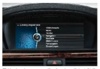
□ Navigation system Professional<sup>3</sup>, incl. DVD drive, iDrive Controller with direct menu control buttons, eight functional bookmarks, integrated hard disk for audio files and navigation data, 3-D map display and high-resolution 8.8" monitor.
