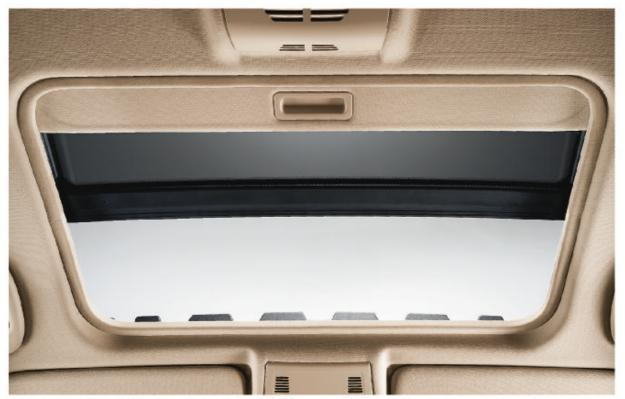
Glass sliding/vent roof, electric, with wind deflector and comfort opening function via the car's remote control unit.
