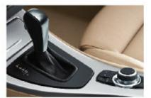
□ 6-speed automatic transmission with Steptronic and ATM (Adaptive Transmission Management). The gearshift mechanism enables very fast, immaculate gear changes – for truly dynamic performance (standard on 335d).
