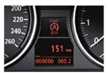
■ Auto Start/Stop display in the Info Display tells you when the engine has been switched off by the Auto Start/Stop function (for example at traffic lights or in a traffic queue). The display is switched off when the engine is restarted automatically (on all four-cylinder models with manual transmission).
