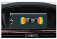
□ Park Distance Control (PDC)<sup>2</sup>, for front and rear or rear only, facilitates the process of parking and manoeuvring in confined spaces, giving you an acoustic signal for the distance between your car and an obstacle. In conjunction with the navigation system<sup>3</sup>, PDC will also provide a visual indication on the monitor display.
