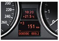
■ Optimum Shift Indicator<sup>1</sup> tells you when shifting to another gear would save fuel. The system indicates whether you should shift up or down and adapts its recommendations to your driving style. When accelerating, for example, the next shift indication comes at the point where a higher gear would enable you to continue accelerating at the same rate, but with reduced fuel consumption.
