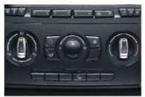
Air conditioning system, incl. microfilter and air recirculation switch, ensures comfortable climatic conditions in the vehicle interior at any time of the year, with manual adjustment of air volume and distribution.
