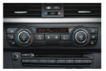
□ Automatic air conditioning, incl. AAR, microfilter, fogging and solar sensors and residual heat button, rapidly provides the desired climatic conditions in the interior and maintains the selected temperature. With individual temperature control at the front (left/ right), air-conditioned storage compartment in the centre console and ventilation and air conditioning for the rear passengers.
