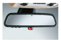
□ Interior mirror, including front reading lights, with automatic anti-glare function and large surface area. The dazzle from following vehicles is automatically reduced when the amount of incident light exceeds a defined limit.
