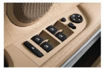
■ Window lifts, electric, front and rear, with open/close toll-booth function, comfort opening/ closing function and trap release on all windows.
