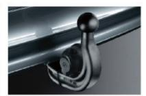
□ **Trailer tow hitch,** incl. trailer stability control, with electric unlocking via a switch in the luggage compartment. If the trailer hitch is not needed, it can be folded away mechanically.
