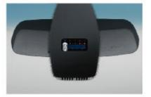
□ Rain sensor with automatic driving lights control: once activated, the rain sensor will automatically switch on the windscreen wipers when it begins to rain, adjusting the wiper frequency in line with rainfall intensity. The integrated automatic driving lights control will switch on the low beam automatically at dusk and in tunnels.
