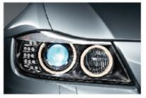
□ Xenon Headlights for high and low beam, incl. LED indicators and automatic headlight range control, provide much better illumination of the road ahead at night or in poor visibility. □ Adaptive Headlights with variable light distribution and turning lights\*, headlights are directed into the bend as soon as the vehicle starts cornering.
