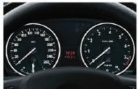
■ Instrument panel with analogue indicators and red backlighting, speedometer with integrated fuel gauge, rev counter with fuel consumption display (on 335i with oil temperature display), digital display for mileage and trip counter, outside temperature display and clock.
