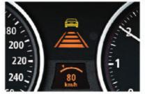
□ Active Cruise Control (ACC) enables comfortable driving at a pre-selected speed. When driving in columns of traffic, your BMW adapts to the speed of a slower preceding vehicle and automatically maintains a pre-set distance (for six-cylinder models only).
