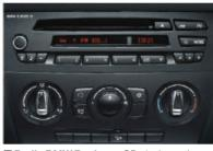
■ Radio BMW Business CD, 4-channel amplifier, aerial diversity, AUX-IN connection, scan function, CD drive, MP3 decoder, automatic volume control, six loudspeakers (four mid-range speakers/tweeters, two central subwoofers under the front seats).
