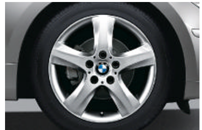
□ BMW light-alloy wheels star-spoke 142 with mixed tyres, 7 J x 17" with 205/50 R 17 tyres at the front, 7.5 J x 17" with 225/45 R 17 tyres at the rear.
