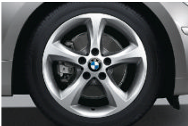
□ BMW light-alloy wheels star-spoke 256 , 7 J x 17", 205/50 R 17 tyres (standard on 130i).
